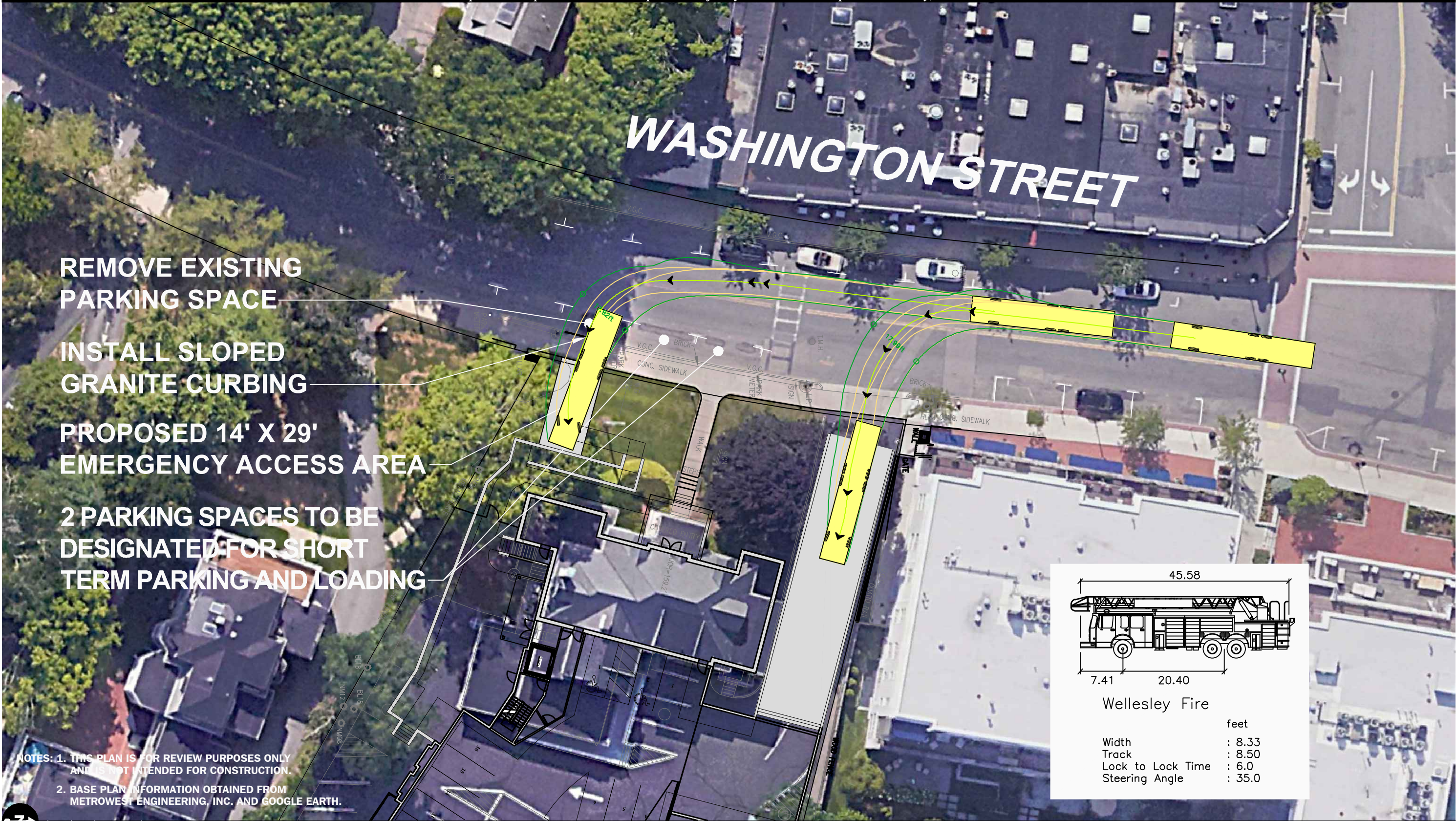
Figure TA-7 Wellesley Fire Truck Entering Garage and Staging Area Turning Analysis
