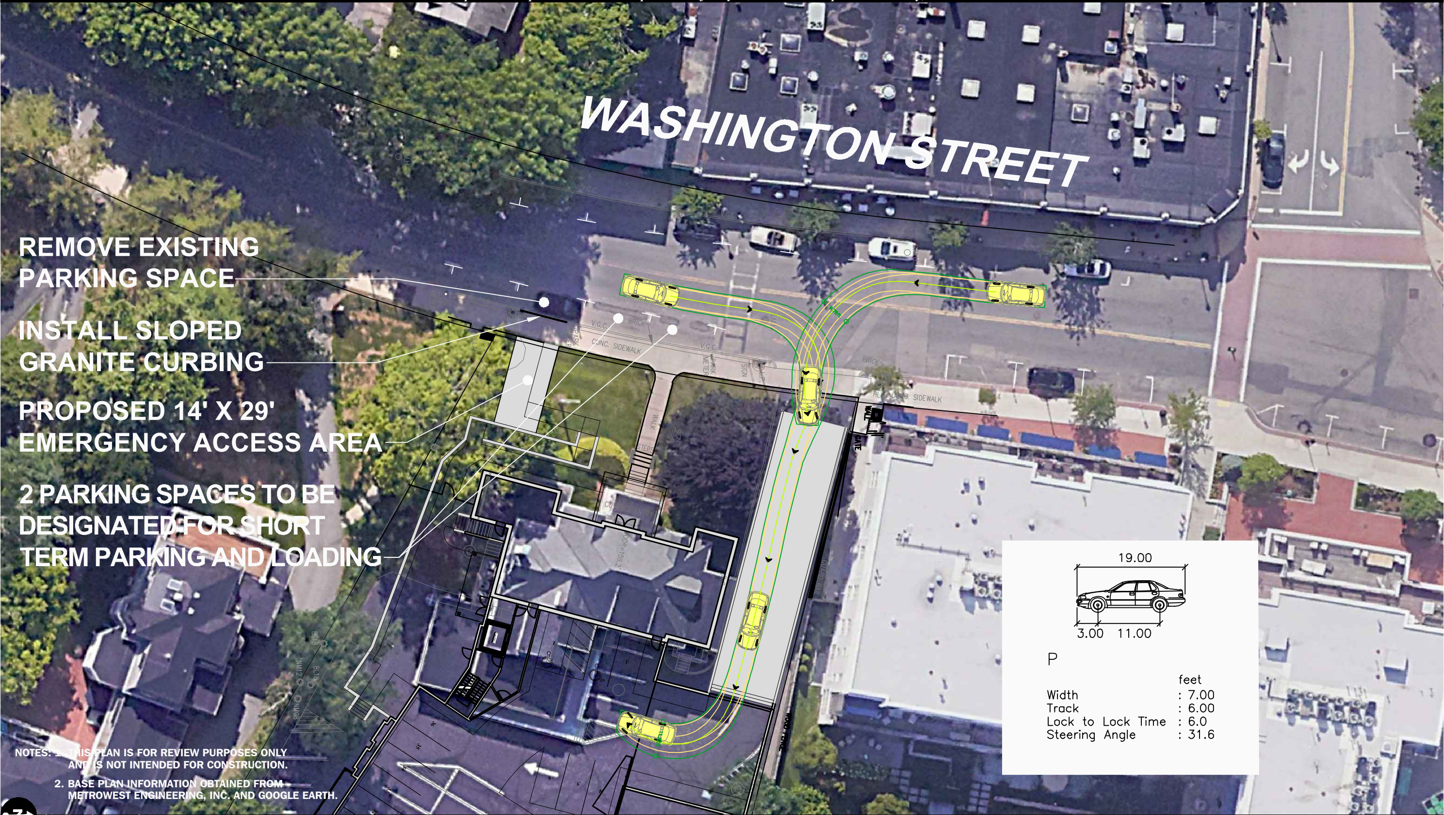
Figure TA-1 Passenger Vehicle Entering Garage Turning Analysis
