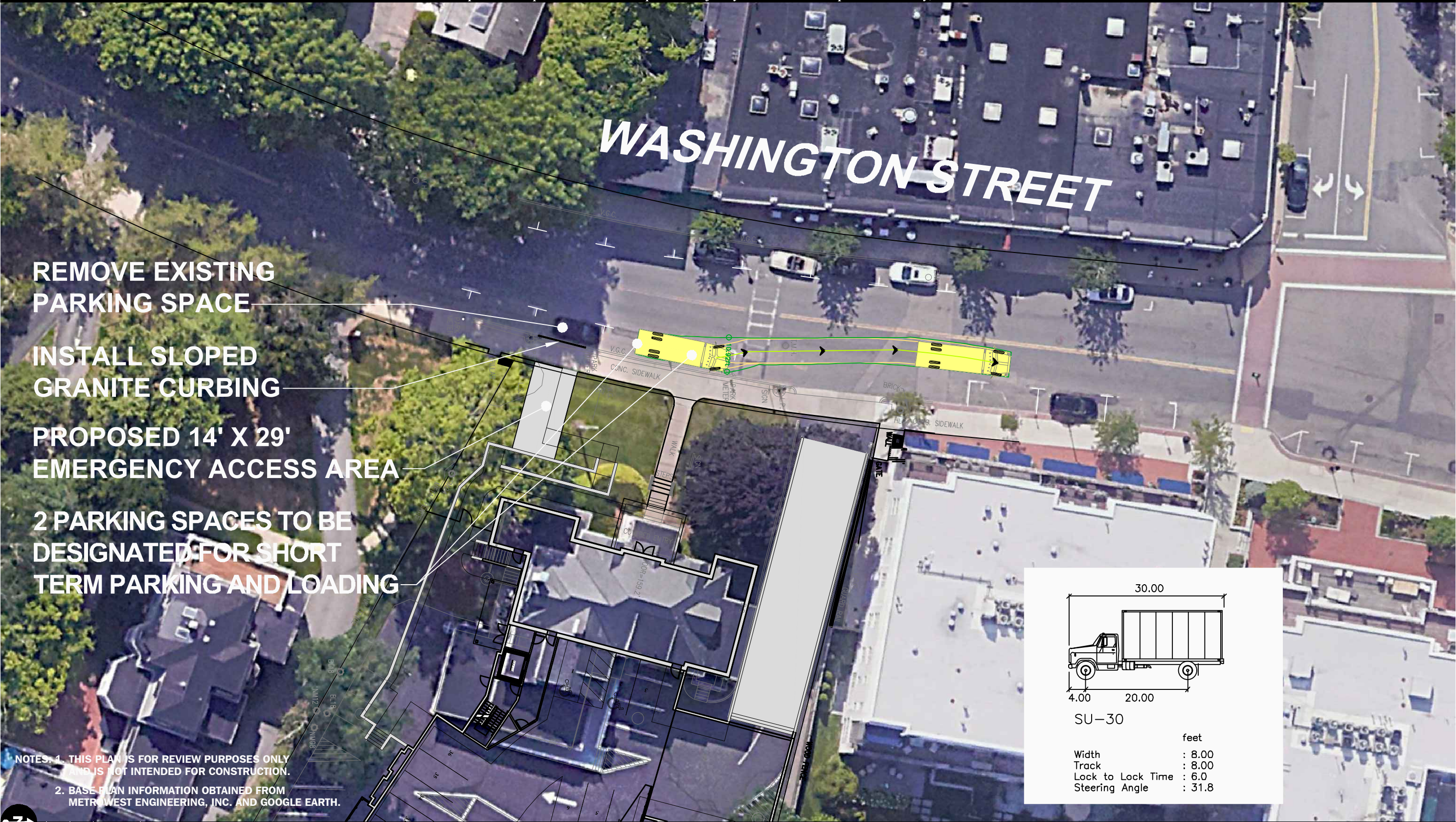
Figure TA-6 SU-30 Exiting Loading Area Turning Analysis
