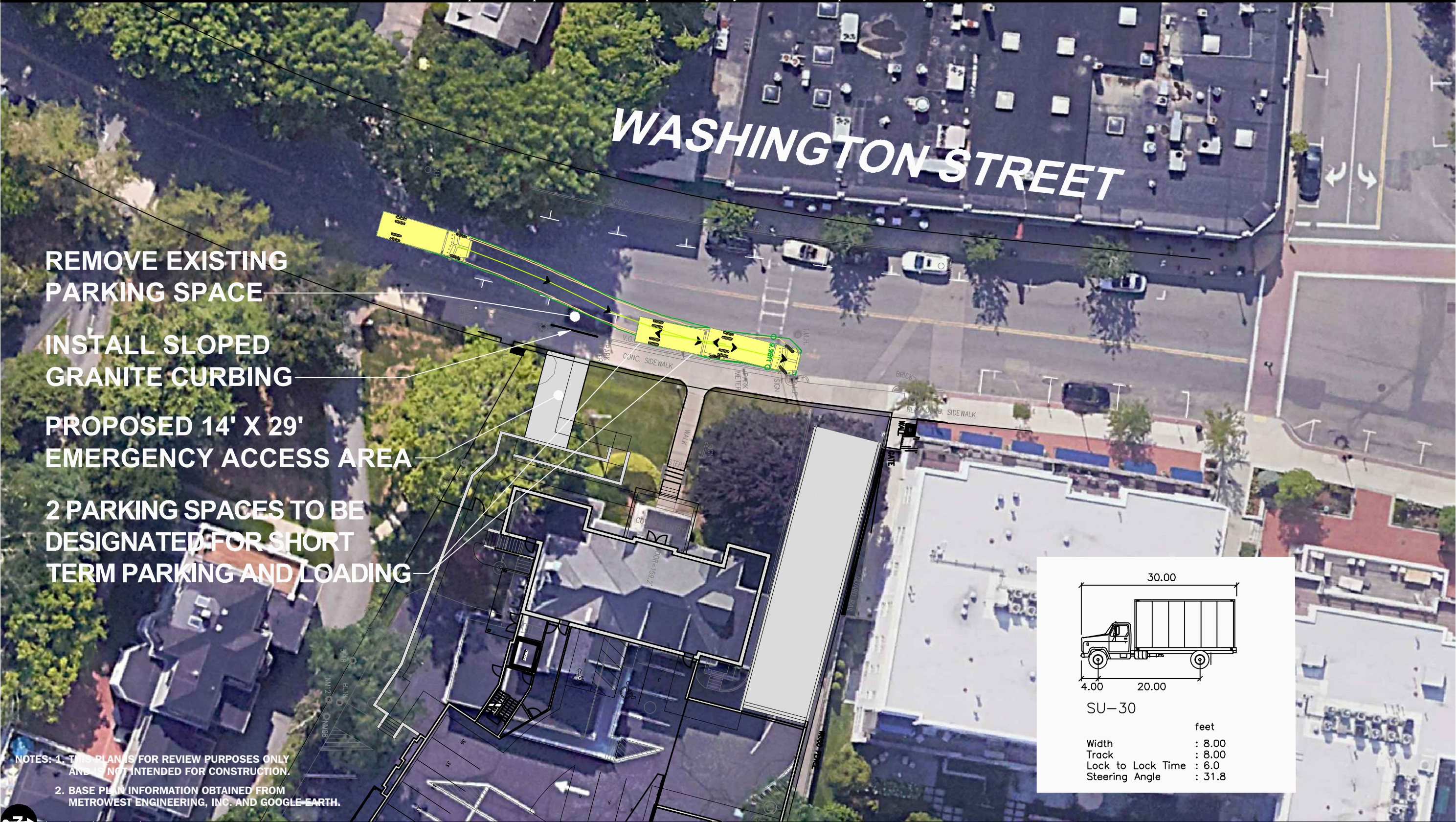
Figure TA-5 SU-30 Entering Loading Area Turning Analysis
