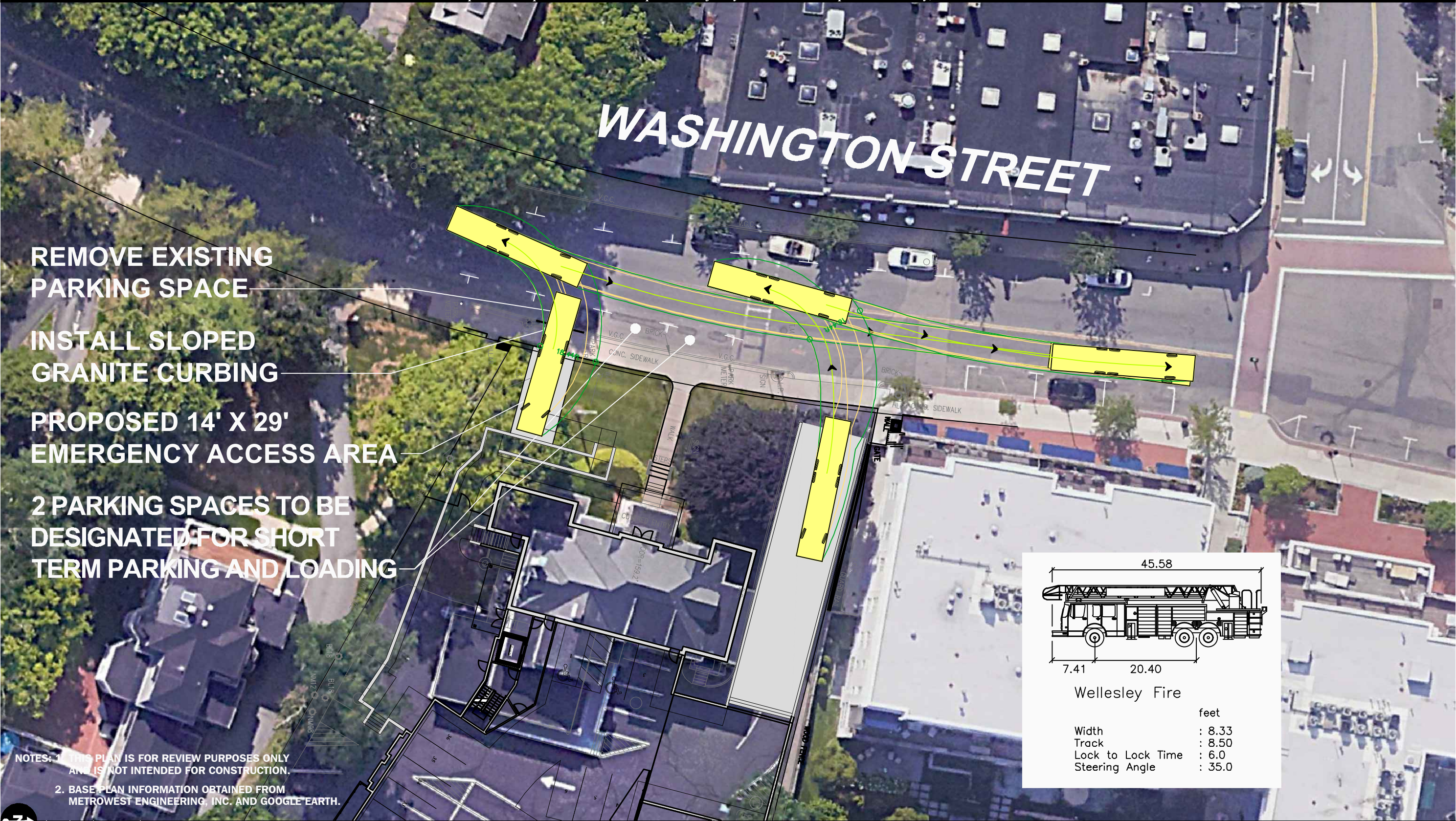
Figure TA-8 Wellesley Fire Truck Exiting Garage and Staging Area Turning Analysis
