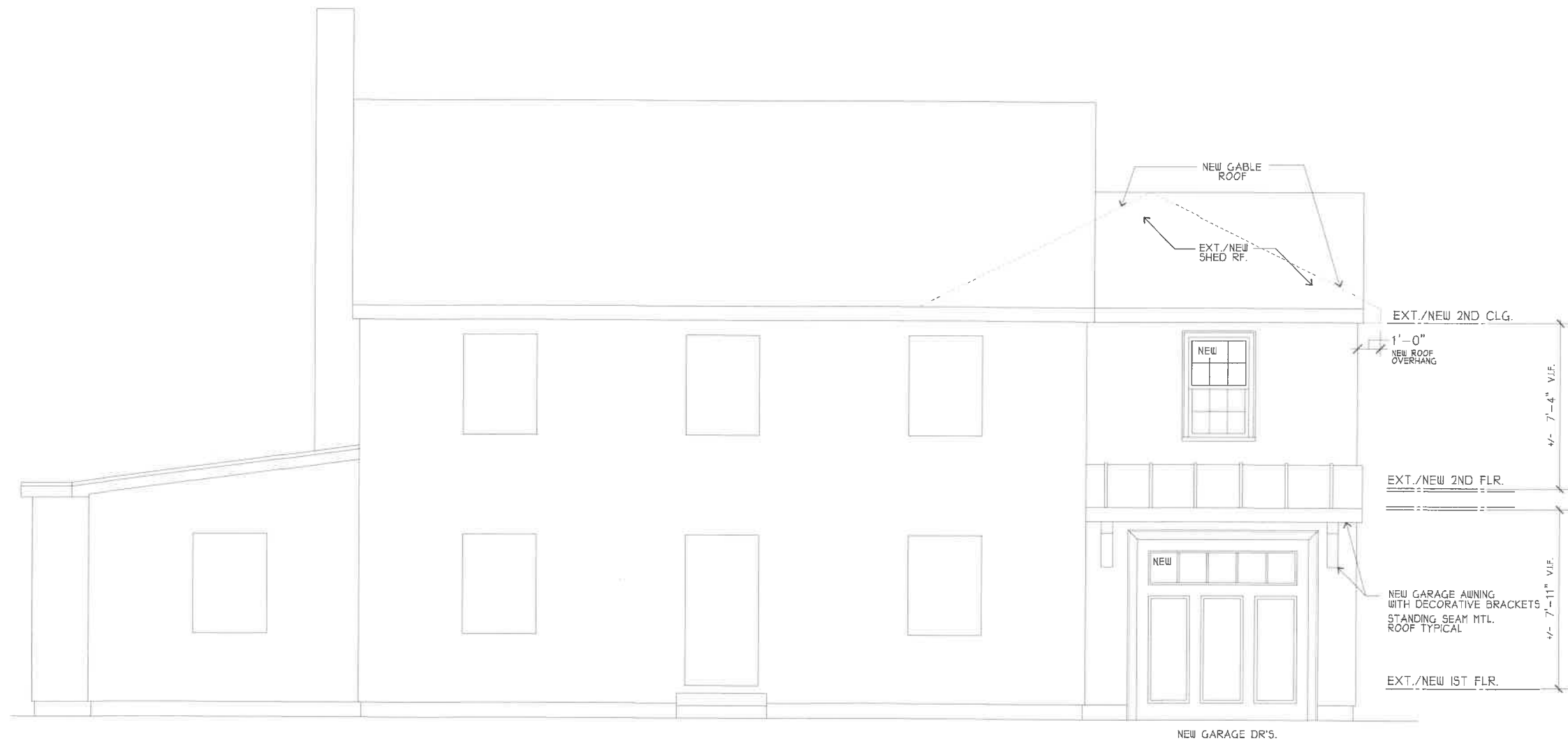
3 EXT./NEW FRONT FACADE ELEVATION SCALE: 3/8" = 1'-0"
