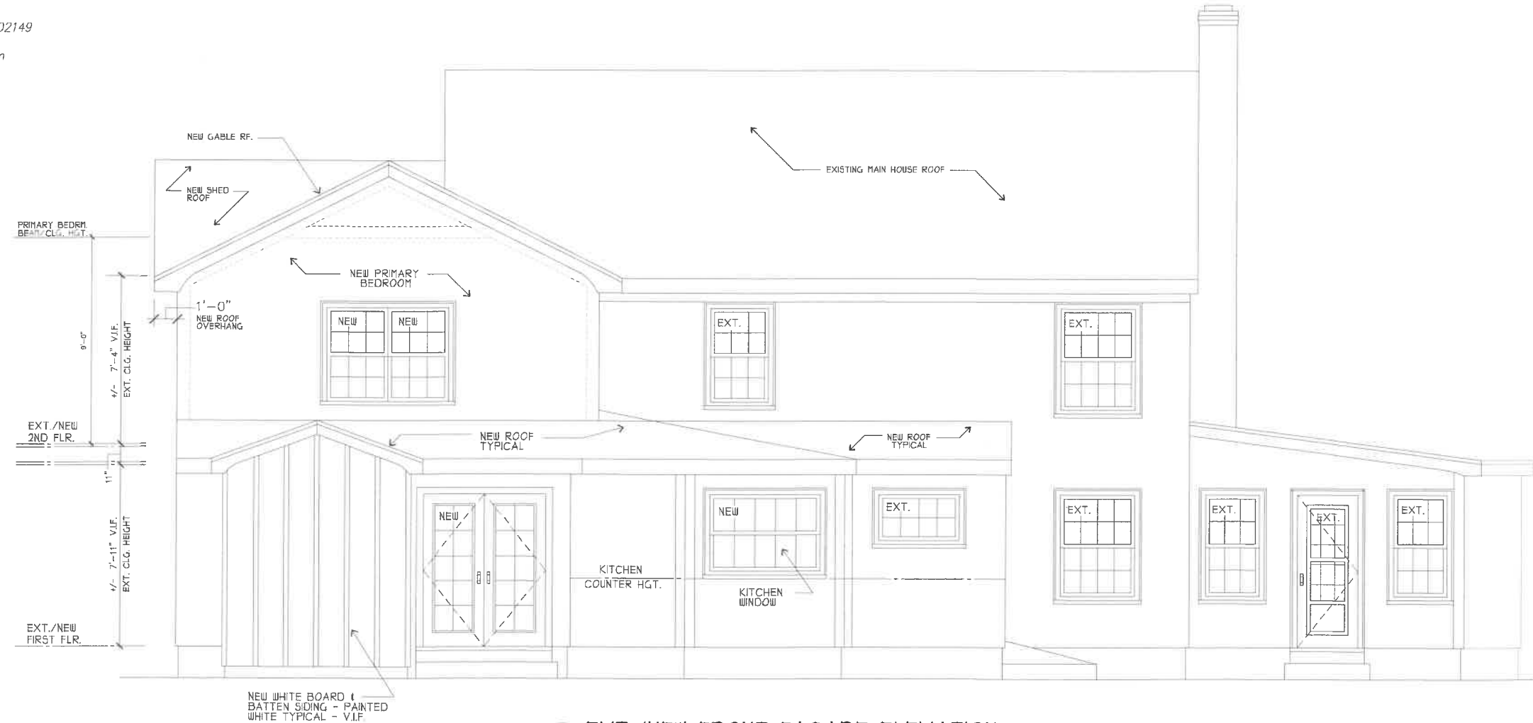
1 EXT./NEW FRONT FACADE ELEVATION SCALE: 3/8" = 1'-0"
