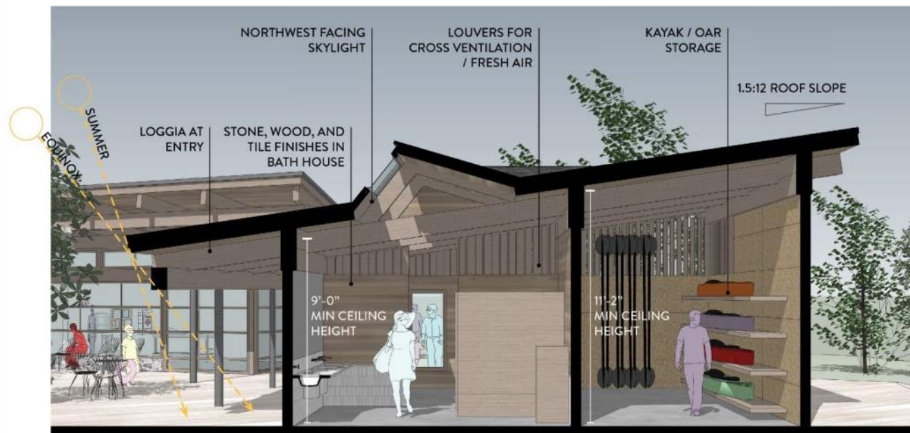
Section through the Bathhouse Building
