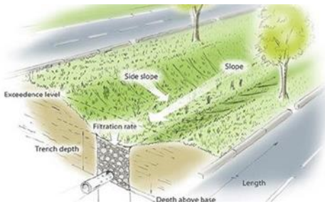
Image: Water quality swale with underdrain. Source: U.S. EPA.
