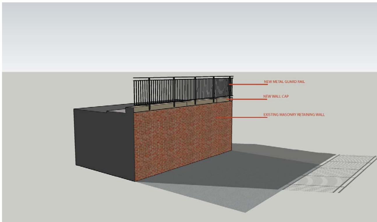
Guardrail - Retaining wall side
